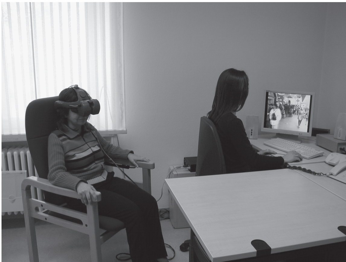
Figure 1 Virtual reality environments are presented using a head mounted display and tracking head movement.
