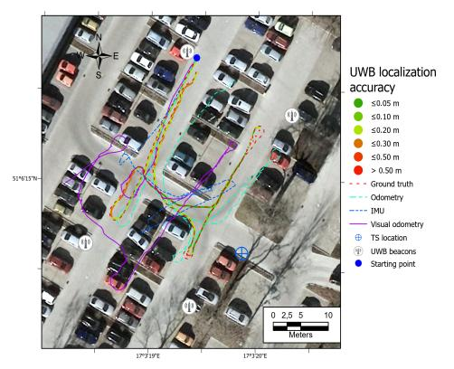
**Figure 12.** Comparison of paths derived from odometry, IMU, UWB, and VO with the ground truth data. Path 1.
