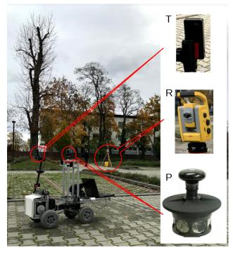
**Figure 5.** Mobile robot equipped with measurement system. T—mobile UWB tag, R—Robotic Total Station (RTS), and P—prism.
