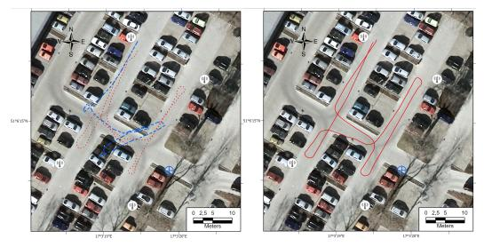
**Figure 20.** Comparison of the IMU-based path recognition method's performance in the case of data acquisition on the non-amortized robot (left-hand side; ground truth drawn as red dotted line) and using an amortized sensor mounted on a robot (right-hand side).
