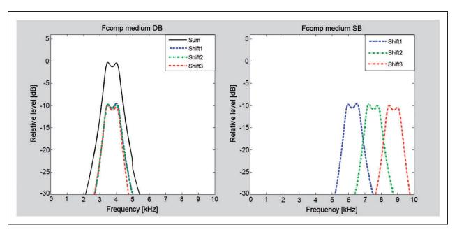
Figure 2. Example of the SB (right panel) and DB (left panel) for the medium setting of Fcomp. Each of the three subbands in the SB (termed "Shift1," "Shift2," and "Shift3" here) is transposed to the same DB. Therefore, the DB is narrower than the SB. Based on information provided by Bernafon AG.
