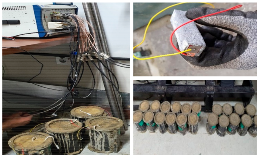
Figure 8. PZT–CNT sensor casting and data acquisition process.
