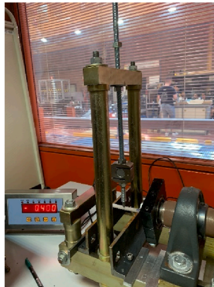
Fig. 24. Machine for bending test.
