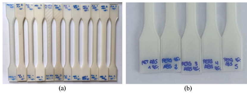
Fig. 15. (a) Tensile specimens. (b) Specimen labeling.
