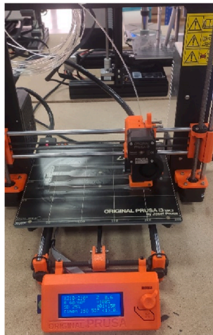
Fig. 5. Prusa i3 MK2S single filament printer.
