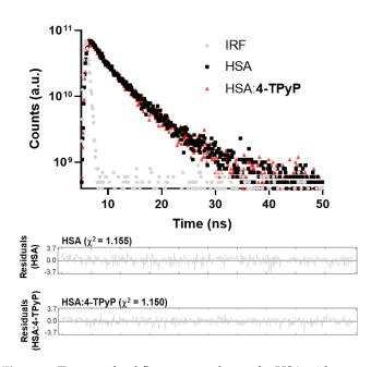
**Figure 3.** Time-resolved fluorescence decays for HSA without and with 4-TPyP at pH = 7.4 and 296 K using an electrically pumped laser (EPL) with an excitation wavelength of  $280 \pm 10$  nm, pulse width of 850 ps, and a typical average power of 1.8  $\mu$ W/pulse, monitoring emission at 340 nm. The residuals correspond to the bi-exponential treatment. [HSA] =  $1.0 \times 10^{-5}$  M and [4-TPyP] =  $1.32 \times 10^{-5}$  M.
