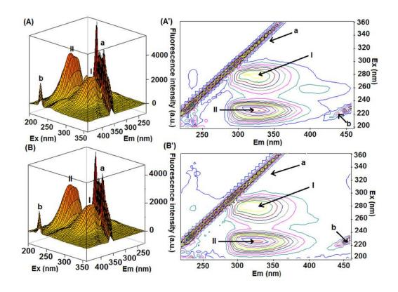
**Figure 6.** The 3D-fluorescence spectra and the corresponding contour maps for (**A**,**A**') HSA and (**B**,**B**') HSA:4-TPyP in pH = 7.4 at room temperature. [HSA] =  $1.0 \times 10^{-6}$  M and [4-TPyP] =  $1.32 \times 10^{-6}$  M.
