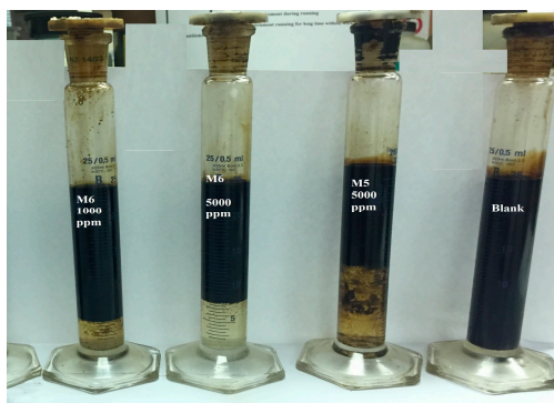
Figure 8. Demulsification photos of petroleum crude oil water emulsions in the presence of M5 and M6 and absence of demulsifier (blank).
