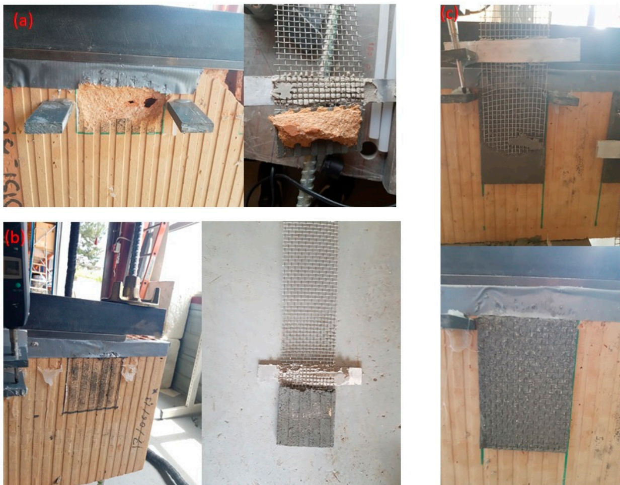
Figure 13. Failure modes of specimens with an anchorage length of (a) 50 mm, (b) 100 mm, and (c) 150 mm.
