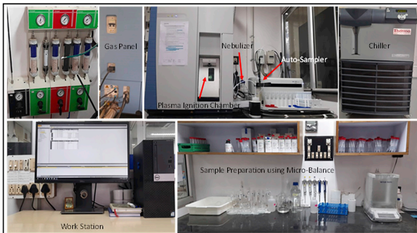
Figure 1. Different parts of ICP-MS instrument and sample preparation demonstration
