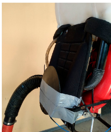
Figure 3. Position of the rubber pad containing the accelerometer, on the padded backrest.
