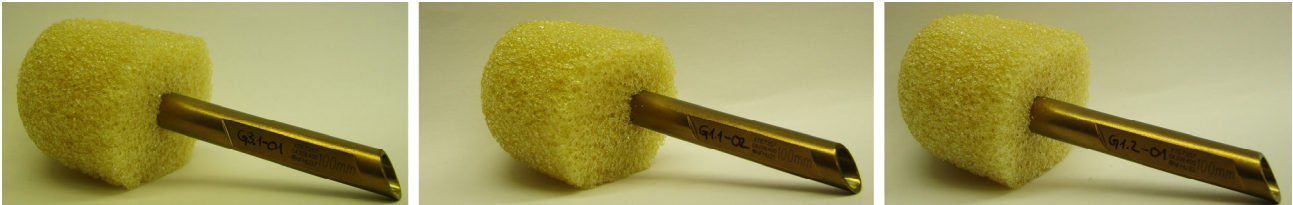
Figure 1. Photographs of surrogate specimens simulating human cancellous bone of right femoral heads implanted with TFN-ADVANCED™ Proximal Femoral Nailing System (TFNA) head elements in central ( left ) and anteroposterior eccentric position with 7 mm anterior ( middle ) and 7 mm posterior ( right ) offset.
