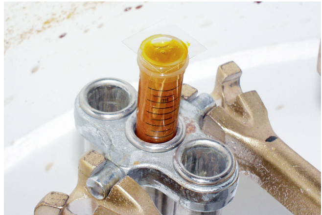
Figure 1-11: Centrifuge with free swinging buckets showing a coverslip in place before centrifugation.
