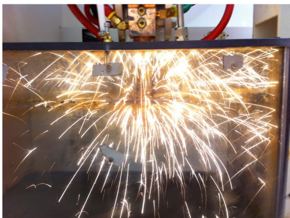
Fig. 2. Images of an active spot weld and generation of sparks.
