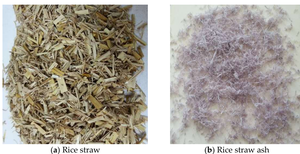
Figure 6. (a) Rice straw and (b) rice straw ash after firing at 950 °C.
