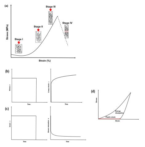
**Figure 2.** (a) Schematic representation of the arrangement of collagen fibres with increasing strain during tensile loading resulting in stiffening. Viscoelastic effects: (b) creep; (c) stress relaxation; and (d) energy dissipation in cyclic loading (only one cycle shown).
