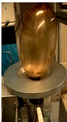
Figure 5. Gelatin films fabricated by blown-extrusion using yucca extract and glycerol. Reproduced with permission from [149].
