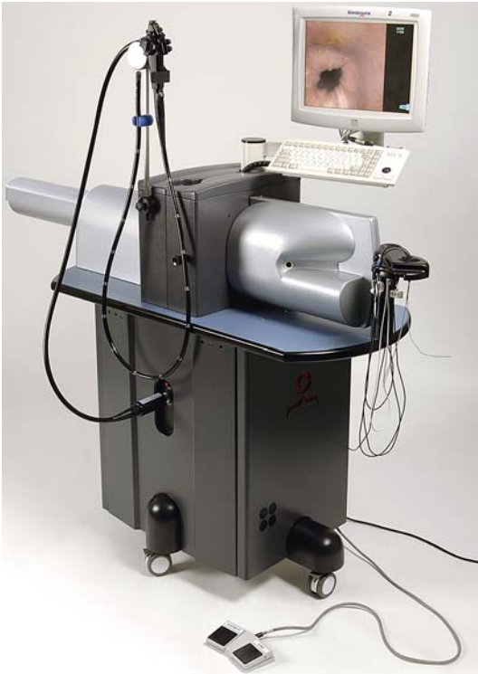
Fig. 1. The GI Mentor II virtual reality simulator, the setup for training in lower endoscopy.
