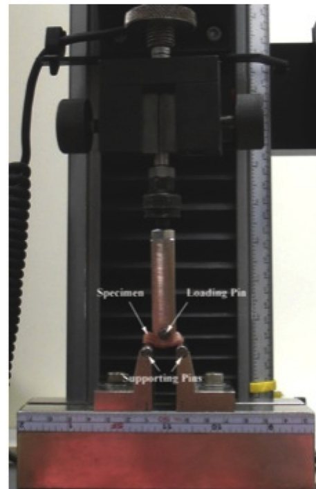
Fig. 2 Photograph showing a test fixture on the Instron testing machine for a three-point bending test. The prepared FU specimen was positioned on the supporting pins with a span of 18 mm, and a loading pin at the mid-point of the span was clamped onto the upper side of the Instron grip. After positioning the construct, an axial compressive force was applied at a constant crosshead rate of 2 mm/min. The deflection of each FU specimen was measured to evaluate the bending stiffness between two FU groups.
