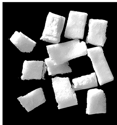
Figure 1. Photograph of the freeze-dried cassava starch foam material, MWB (microwaved for 20 s).
