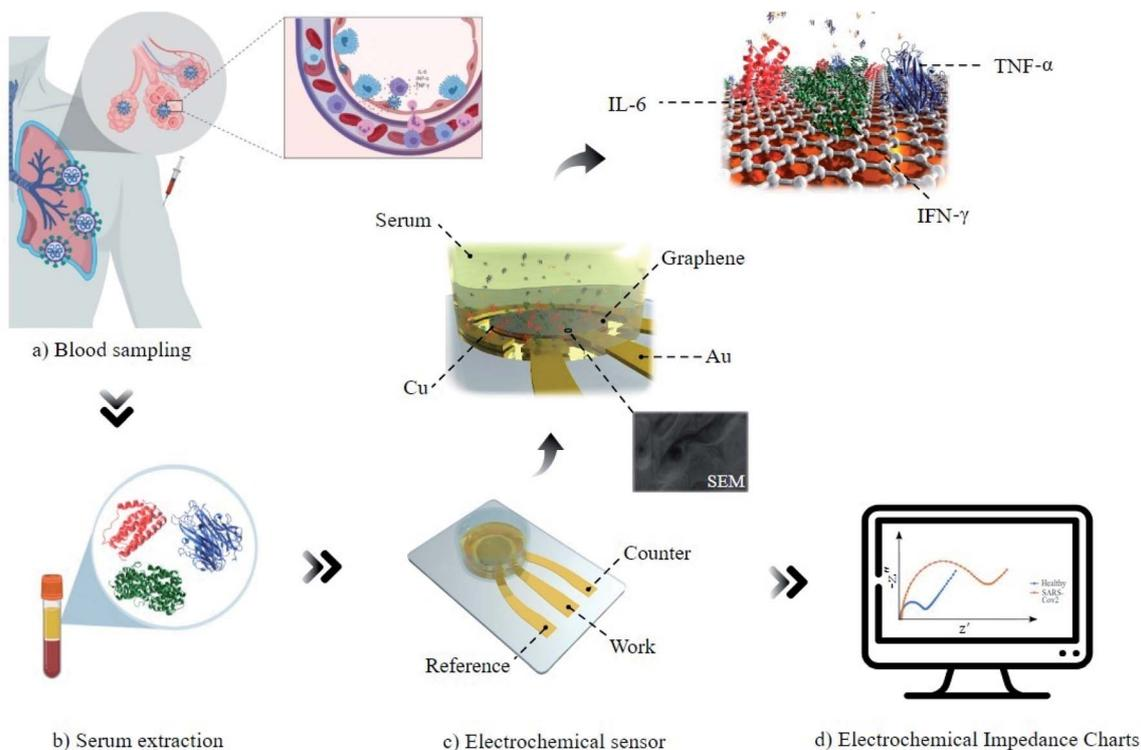
**Fig. 3** Schematic diagram of the procedure of cytokine storm diagnosis in patients suspected to have COVID-19 by the EIS method. Blood is sampled from the normal donors and different stages of patients and then the serum is isolated and mixed with the electrolyte. The mixed solution is then added to the three-electrode system with graphene/Cu WE and at the end EIS is performed and  $R_{CT}$  is extracted for each sample.
