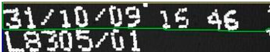
Figure 12. A divider is capable of separating two lines even though there are no rows with zero ink.
