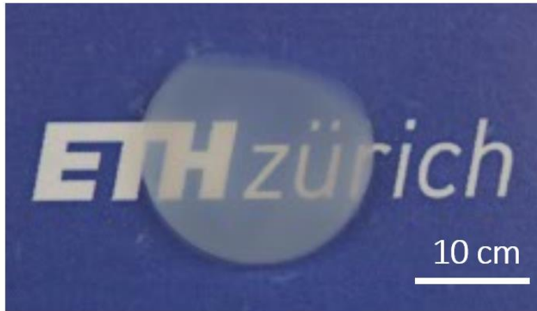
Figure S12. Hydrogel synthesized from oat globulin amyloid fibrils. The semi-transparent hydrogel was cross-linked by mixing the amyloid fibril solution with an NaCl solution at a final concentration of 450 mM and was dialyzed through a semi-permeable membrane for 2 days.
