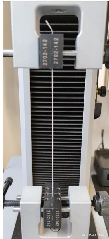
**Figure 2.** A dental floss sample loaded onto the tension testing system. The bottom part is fixed and the top part connected to a force transducer, and movable. In this case, straight, rubberized fixtures were used to avoid floss slippage.
