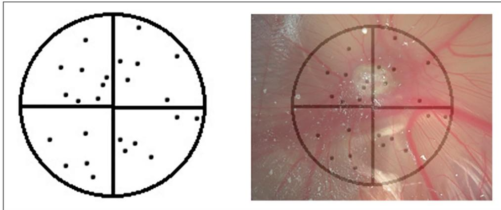
**Figure 6.** Example drawing of a Chalkley graticule eyepiece showing the layout of dots to align over blood vessels, allowing counting to quantify the angiogenic response to materials, such as BMP-2 soaked collagen sponge shown.
