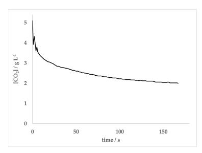
**Figure 5.** Time-dependent kinetics of CO<sub>2</sub> escape from 500 g of a solution containing 4.84 g L<sup>-1</sup> of CO<sub>2</sub> and 5% by mass ethanol at 20 °C and P<sub>atm</sub> = 0.992 bar. The reaction was initiated by the addition of a single Mentos candy at t = 0 s.
