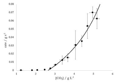
**Figure 4.** Rates of degassing from 5% by mass solutions of ethanol in water at 20 °C and  $P_{atm} = 0.975$  bar. Degassing was initiated by addition of a single Mentos candy. Error bars represent 95% confidence interval.
