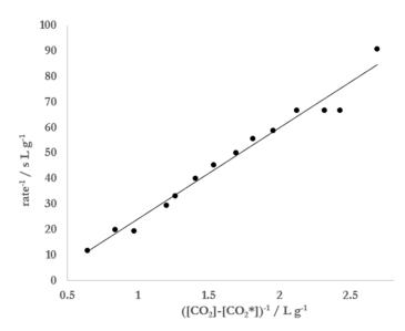
**Figure 6.** Inverse of the rate of degassing vs. the inverse of  $([CO_2] - [CO_2^*])$  for a 5% by mass solution of ethanol in water. The data presented here represent data from Figure 4 from t = 3 to 17 s. The best linear fit to these data was achieved ( $R^2 = 0.97$ ) when  $[CO_2^*] = 2.77$  g L<sup>-1</sup>.
