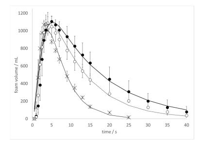
**Figure 3.** Kinetics of foam production when 1 min Mentos candy is added to 500 mL of Diet Coke at 20–21 °C as described in the text. (**Closed circles**) Control samples to which water was added; (**open circles**) samples to which 0.5 %; and (**X's**) 5% ethanol by mass was added. Lines represent fits to the data using parameters listed in Table 1. Error bars represent one standard deviation.
