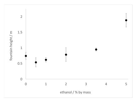
**Figure 2.** Fountain heights achieved when 2 L of Diet Coke is treated with increasing amounts of ethanol as indicated in the text and then 11 mint Mentos are added at 20–21 °C. Error bars represent one standard deviation.
