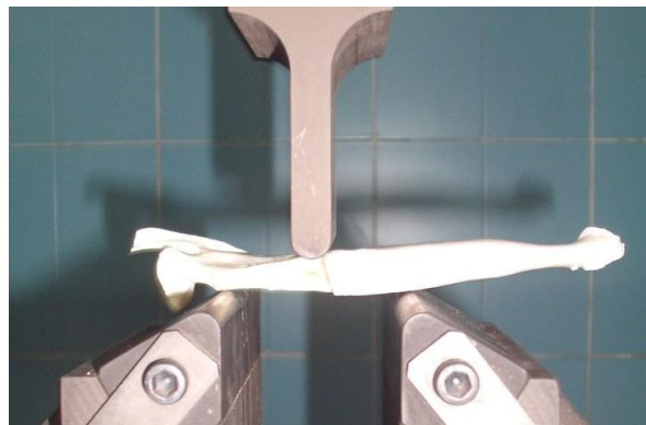
Figure 1 Three points bending test applied on the goat mandible.
