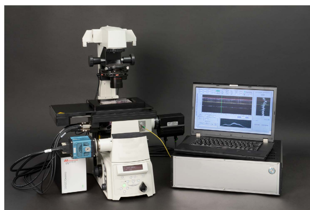
Figure 2. Implementation of the high-speed microscopy solution with the OCT-based autofocus system on an inverted Nikon Ti-E microscope. The fibre of the focus measurement system is coupled into the microscope using a modification on the fluorescence port. See also the dotted line in the drawing of Fig. 4a. Coupling via the camera port is shown in Fig. 4b.
