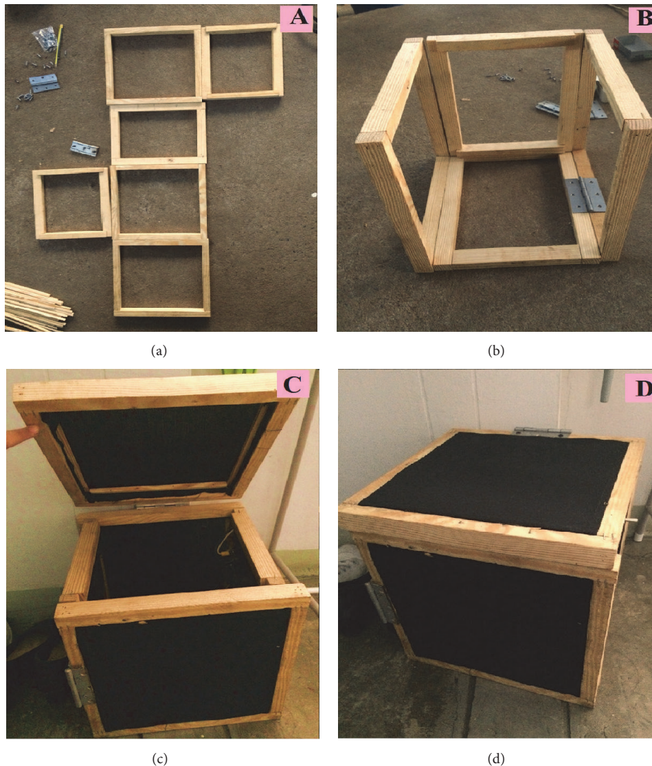
FIGURE 2: Design of the mosquito trapping box tested in Step 2 of the research and development phase. (a) A wooden frame was constructed using tacks; (b) the wooden frame was then used to make a square box with an opening lid for mosquito removal; (c) black cotton cloth was attached to the wooden frame; (d) appearance of the final wooden trapping box combined with black cotton cloth.
