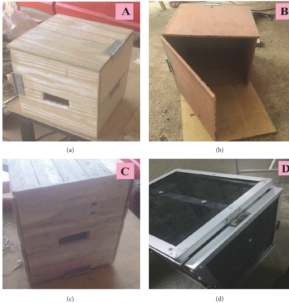
FIGURE 1: Design of the mosquito trapping boxes tested in Step 1 of the research and development phase. (a) Wooden trapping box constructed from Pinus kesiya wood; (b) wooden trapping box constructed from Dipterocarpus alatus wood; (c) wooden trapping box constructed from Tectona grandis wood; (d) control trapping box constructed from aluminum and black plastic mesh.
