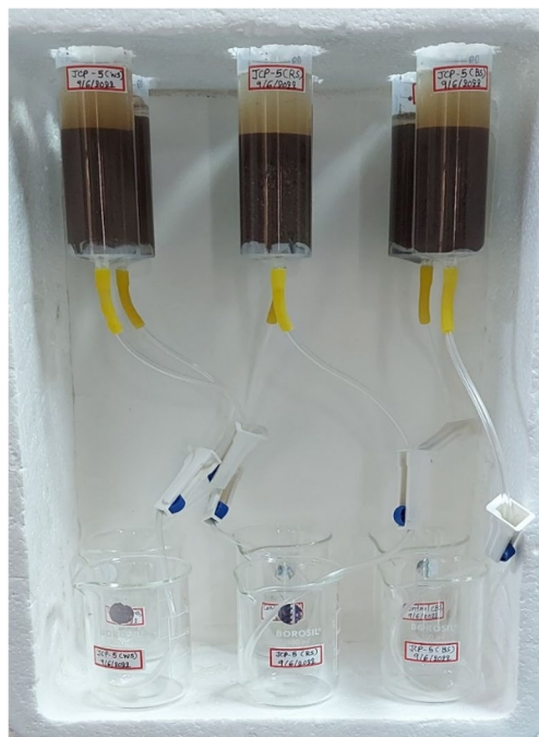
Figure 1. Setup for sand solidification test.
