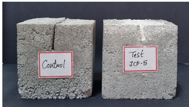
Figure 11. Crack remediation experiment.
