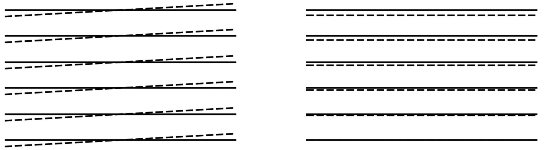
Figure 2. Elementary distortions of the stripes. Rotation (left) and compression (right) of the stripes away from their equilibrium positions indicated by the solid lines.
