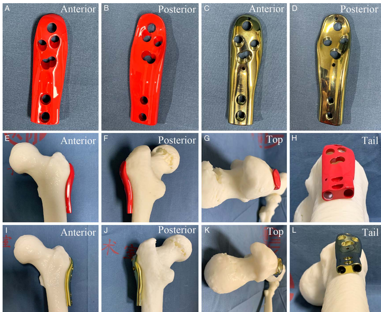
Figure 6. End-structure of anatomical proximal femoral locking plate of three-dimensional printing (A and B) and titanium alloy (C and D). Good match was achieved between proximal femur and end-structure in three-dimensional printing model (E, F, G, and H) and titanium alloy model (I, J, K, and L).
