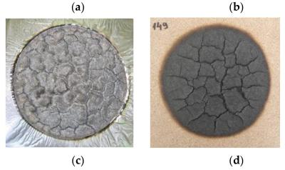
**Figure 4.** Combustion process of particleboards after their ignition by radiant heat (**a**) top view for sample with 15 mm thickness immediately after experiment; (**b**) side view for sample with 15 mm thickness immediately after ignition; (**c**) sample with 15 mm thickness taken out from the measuring device, placed at a distance of 20 mm after the end of the experiment; (**d**) cooled sample 10 min after the experiment, sample thickness of 18 mm.
