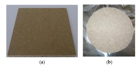
Figure 1. Example of experimental samples. (a) Particleboard; (b) sample prepared for measurements in accordance with ISO 5657 [34].
