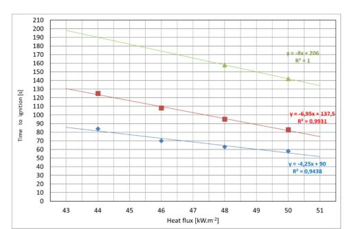
**Figure 11.** Graphical dependence of the time to ignition on the heat flux (44, 46, 48 and 50 kW·m<sup>-2</sup>) and the distance of the particleboard with thickness of 12 mm from the ignition source. Legend: blue-20 mm; red-40 mm and green-60 mm.
