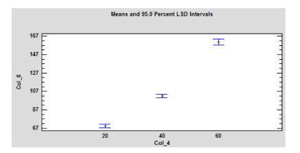
**Figure 12.** Graphical representation of the statistical evaluation-the influence of the sample position and heat flux on the time to ignition source on the particleboards. Legend: Col\_4-position of the sample i.e., distance of the sample from the source; Col\_6-time to ignition. The values are statistically significant at  $p \le 0.05$  according to LSD ANOVA.
