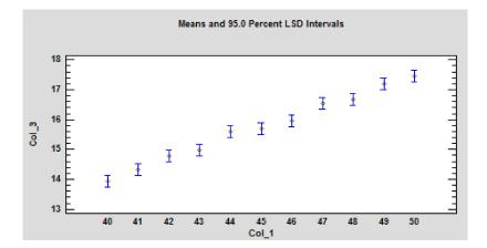
**Figure 9.** Graphical ANOVA for mass loss (Col\_3). Legends: Col\_1 is heat flux; Col\_2 is thickness of particleboard samples as the variance of the values shown in blue. The values are statistically sig-nificant at  $p \le 0.05$  according to LSD ANOVA.
