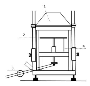
**Figure 2.** Scheme of the equipment for determination of flammability of materials at a heat flux of radiant heat of 10–50 kW·m<sup>-2</sup> according to ISO 5657: 1997 [34]. Legend: 1-heating cone, 2-board for sample, 3-movable arm, 4-connection point for recording experimental data.
