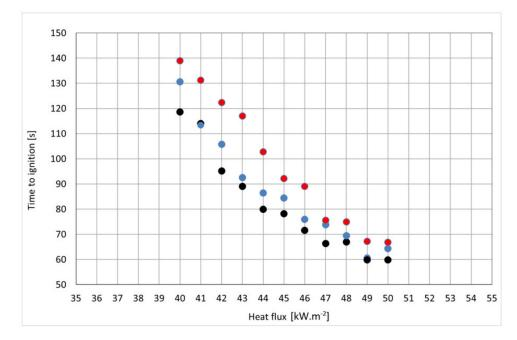
**Figure 6.** Graphical dependence of the time to ignition on the heat flux and thickness of the particleboard. Legend: black point-12 mm thickness; blue point-15 mm thickness; red point-18 mm thickness.
