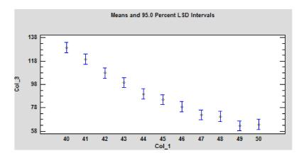
**Figure 7.** Graphical representation of the statistical evaluation-the influence of the sample thickness and heat flux on the time to ignition under the action of the radiant heat source on the particleboard. Legend: Col\_1-heat flux; Col\_2-thickness of particleboard samples as the variance of the values shown in blue; Col\_3-Time to ignition. The values are statistically significant at  $p \le 0.05$  according to LSD ANOVA.
