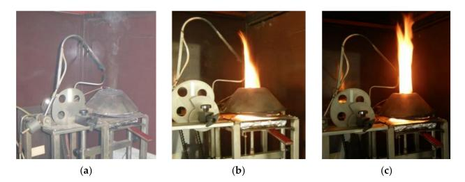
**Figure 3.** Course of measurement of time to ignition and weight loss for a particleboard sample with a thickness of 15 mm, heat flux intensity 45 kW·m<sup>-2</sup>. Legend: (a) sample ignition (time to ignition 84 s); (b) burning of the sample in 100 s; and (c) burning of the sample in 120 s.
