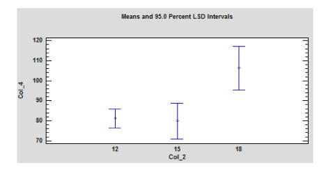
**Figure 5.** Graphical dependence of the ignition temperature on the thickness of the particleboard. Legend: axis "y"-Col\_4 istime to ignition, axis "x"-Col\_2 is thickness for heat flux interval <43,48> kW·m<sup>-2</sup>. The values are statistically significant at  $p \le 0.05$  according to LSD ANOVA.
