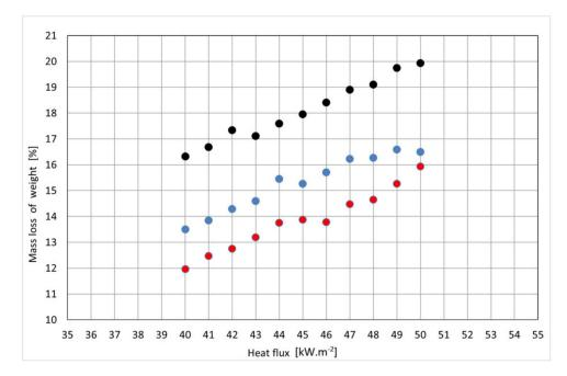
**Figure 8.** Graphical dependence of average values of weight loss on heat flux and particleboard thickness. Legend: black point-12 mm thickness; blue point-15 mm thickness; red point-18 mm thickness.
