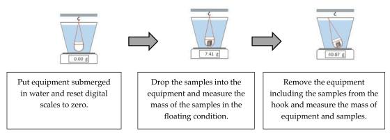
Figure 4. Schematic of the underwater weighing test.
