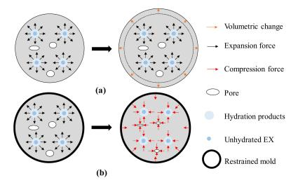
**Figure 8.** Schematic of the effect of chemical stress on the pore structure: (**a**) free condition and (**b**) triaxial restrained condition.
