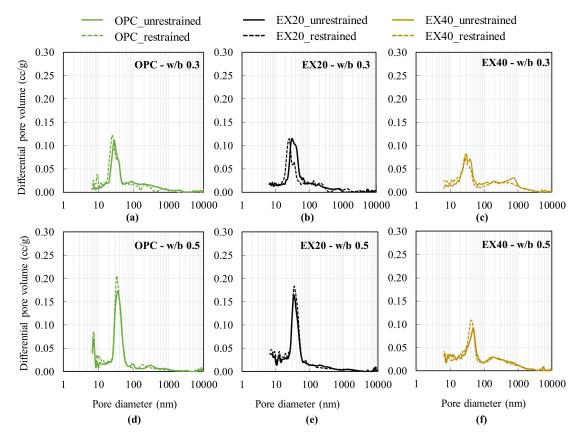
**Figure 7.** Effect of the triaxial restrained condition on the pore size distribution of the cement and expansive mortar under the restrained and unrestrained conditions with different w/b ratios: (**a**–**c**) test results of OPC, EX20, and EX40 with w/b 0.3, respectively; and (**d**–**f**) test results of OPC, EX20, and EX40 with w/b 0.5, respectively.
