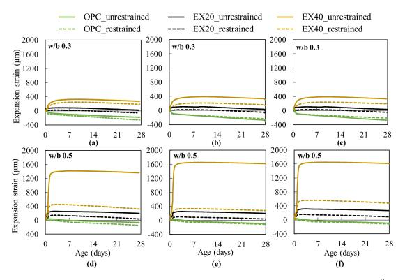
**Figure 6.** Expansion strain of concrete: (**a**,**d**) test results of the sample measuring  $75 \times 75 \times 400 \text{ mm}^3$ ; (**b**,**e**) test results of the sample measuring  $100 \times 100 \times 400 \text{ mm}^3$  (free standard); and (**c**,**f**) test results of the sample measuring  $100 \times 100 \times 400 \text{ mm}^3$  (JIS A 6202 [4]).
