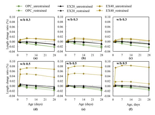
**Figure 5.** Length change ratio of concrete: (**a**,**d**) results of the sample measuring  $75 \times 75 \times 400 \text{ mm}^3$ ; (**b**,**e**) results of the sample measuring  $100 \times 100 \times 400 \text{ mm}^3$  (free standard); (**c**,**f**) results of the sample measuring  $100 \times 100 \times 400 \text{ mm}^3$  (JIS A 6202).
