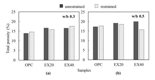
**Figure 9.** Relationship between the total porosity and EX contents under the unrestrained and triaxial restrained conditions: (**a**) w/b ratio of 0.3 and (**b**) w/b ratio of 0.5.
