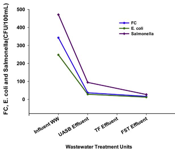
Figure 5. Mean levels of microbial loads at the various treatment units.
