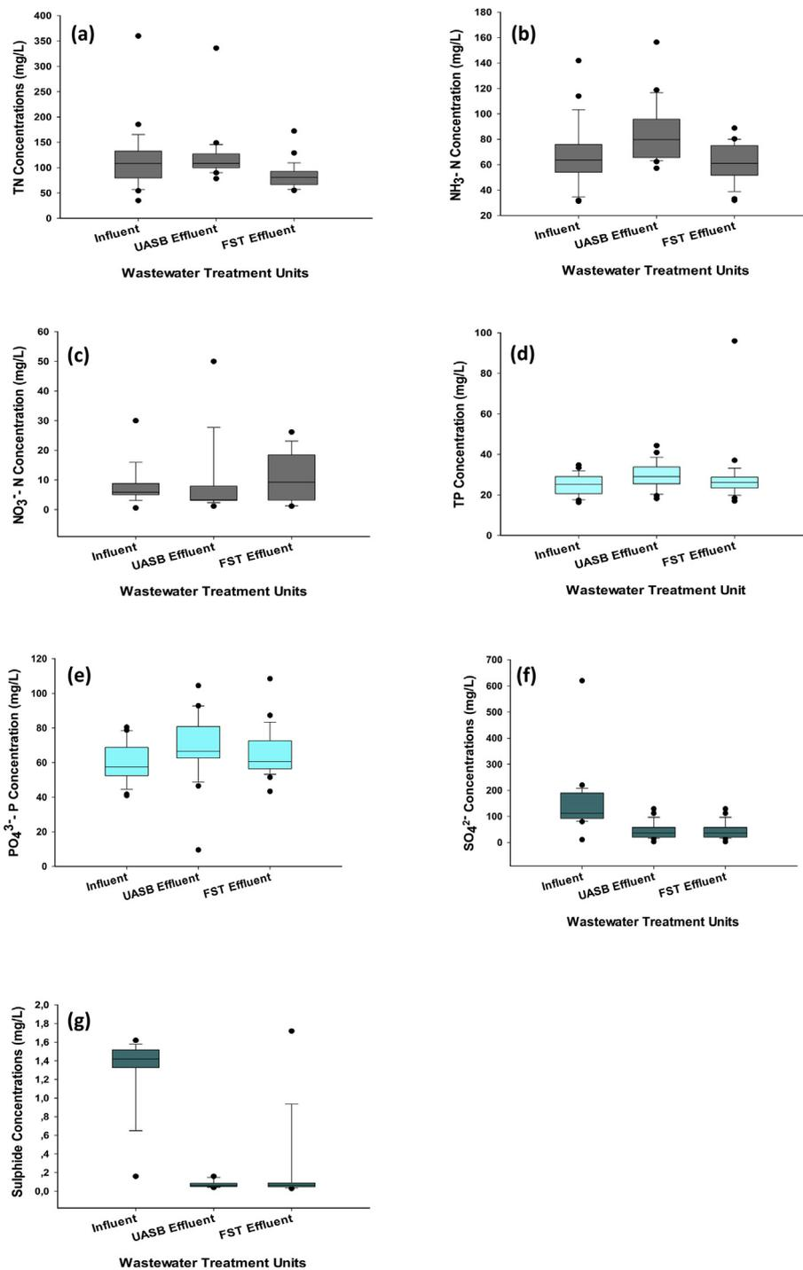
Figure 4. Sewage nutrient concentrations: (a) TN, (b) NH<sub>4</sub>-N, (c) NO<sub>3</sub>-N, (d) TP, (e) PO<sub>4</sub>, (f) Sulphide, and (g) SO<sub>4</sub><sup>2-</sup> at the various treatment units.
