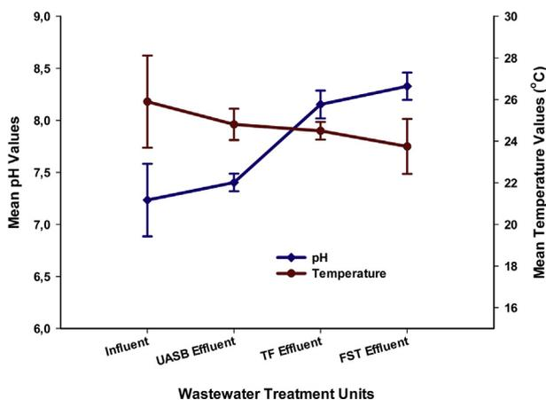
**Figure 2.** pH and temperature variations at the various stages of the treatment process.
