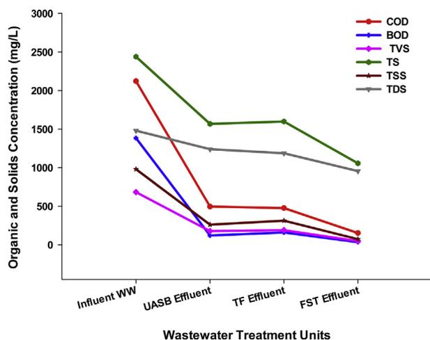
**Figure 3.** Mean concentrations of solids and organic loads at the various treatment units.
