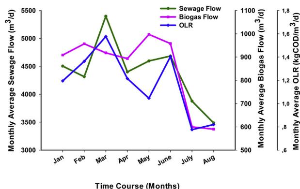
Figure 6. Variations in OLR, sewage and biogas flows.
