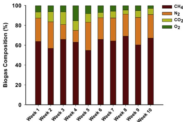
Figure 7. Biogas composition.
