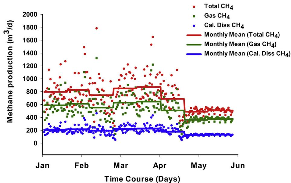
Figure 8. Comparison of total, gaseous and calculated dissolved methane
