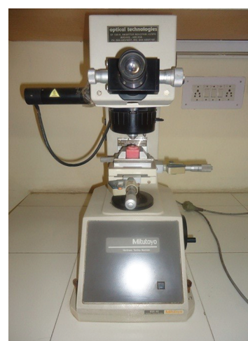
Fig. 5: Vickers microhardness tester
