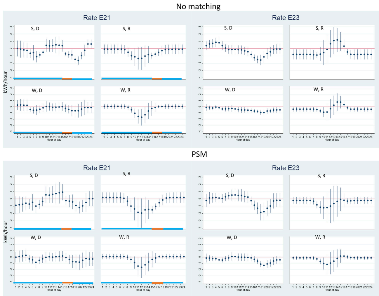
Figure 3. Impact of battery adoption on electricity delivered (purchases) or received (exports), rate plans E21 (5 consumers) and E23 (12 consumers)
