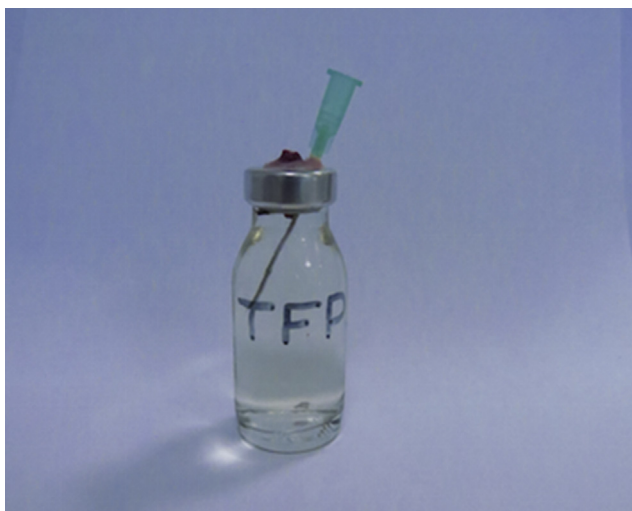
Figure 1 A sample embedded and fixed into a glass vial filled with brain–heart infusion broth through the rubber stopper of the vial. Needle was inserted into the rubber stopper to equalize the pressure.
