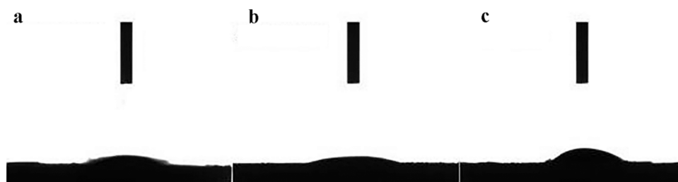
Figure 3. Contact angle: (a) sol-gel-modified electrode material; (b) thermal-modified electrode material; and (c): unmodified electrode material.
