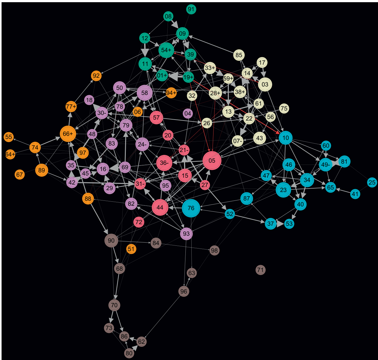
Fig. 2. IC network graph. Network graph visualization of the IC network using the ForceAtlas-algorithm (gephi.org), with edge thickness for partial correlations ( r > 0.02 – 0.29 ) grey color for positive correlations, red color for negative correlations. Node color for modularity (see Table 1). Node size for betweenness centrality. Nodes were automatically assigned coordinates based on a force-directed layout algorithm which treats nodes as positive charges that repulse each other, while being constrained by their links.
