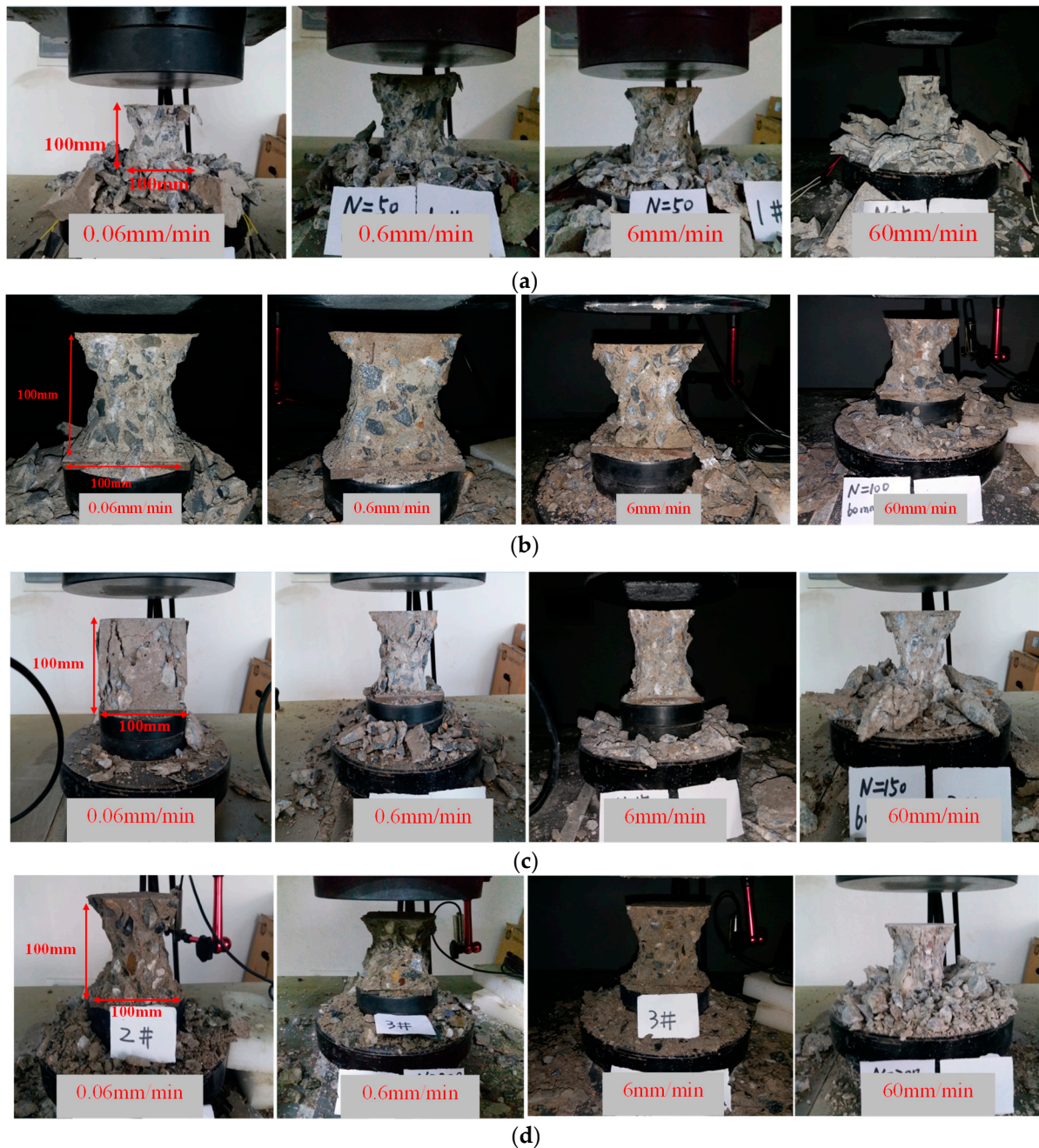
Figure 12. Failure modes with different strain rate and freeze–thaw cycles. (a) 50 freeze–thaw cycles, (b) 100 freeze–thaw cycles, (c) 150 freeze–thaw cycles, (d) 200 freeze–thaw cycles.
