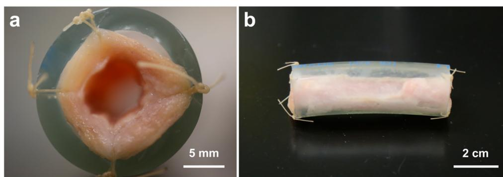
**Figure 2.** Photograph of the pig’s urethra inside a tube. (a) Front view of the pig urethra inside the tube. (b) Side view of the urethra tube with a length of 7 cm.
