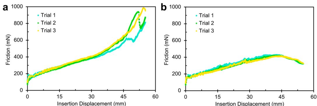
**Figure 5.** Sliding friction during catheter insertion, showing the variation across three trials on the same pig urethra. (a) For the uncoated (U) PVC catheter, the maximum friction increased from trial to trial. (b) In contrast, the lubricant-impregnated catheters show minimal trial-to-trial variation in maximal sliding friction, as shown here for the LIS-10 catheter.
