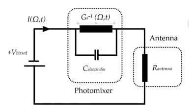
Figure 2. Equivalent circuit of photomixer based THz antenna.
