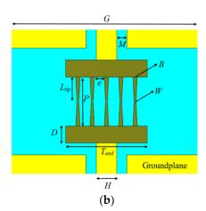
Figure 3. (a) Configurations of the 2D-PhC unit cell; (b) Top view of the photomixer based slot.
