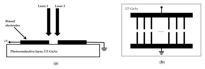
Figure 1. (a) Typical photoconductive photomxing scheme; (b) Top view of photomixer electrodes.
