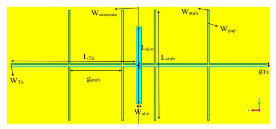
Figure 8. Top view of feeding slot and CPS.
