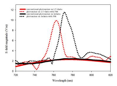
**Figure 5.** Optical E-field magnitude between the central electrodes of a photomixer on the surfaces of LT-GaAs and I GaAs photoconductive layers.
