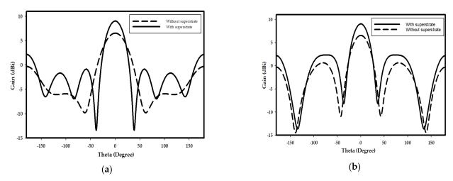
**Figure 11.** Radiation pattern of DRA with and without superstrate at (a)  $\varphi = 0^{\circ}$ ; (b)  $\varphi = 90^{\circ}$ .
