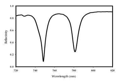
Figure 4. Reflectivity of the 2D-PhC FSS.
