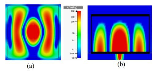
Figure 10. The H-field component inside the DRA with TE<sub>711</sub>mode at (a) XY plane; (b) XZ plane.
