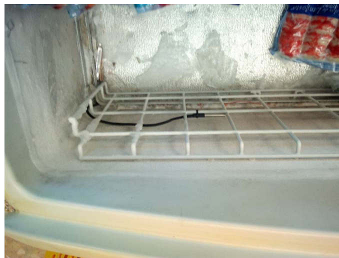
Figure 7. DS18B20 probe placed in a freezer for the experimental setup.
