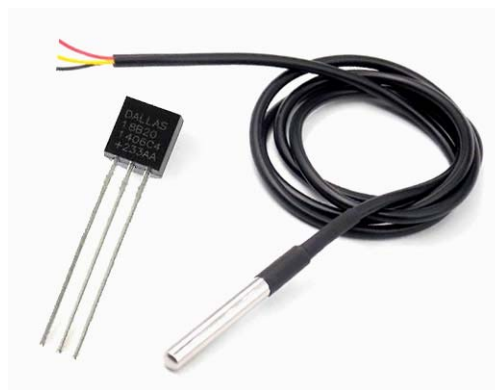
Figure 5. Sensor DS18B20 with TO-92 enclosure (left) or sealed stainless steel sheath (right).
