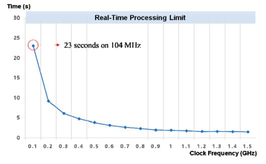
**Figure 6.** Performance of the real-time processing for sleep stage classification. The inference speed with O = 7, I = 14, W = 800 according to the clock frequency of the CPU core.
