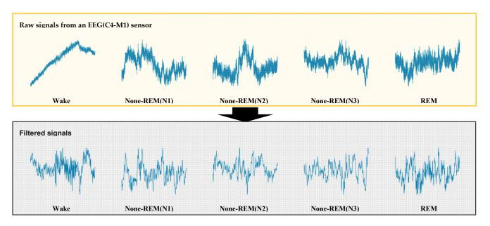
**Figure 1.** Representative raw data sample from each sleep stage. Bandpass filtering was applied to raw polysomnographic data to reduce impact of noise and for artifact reduction.
