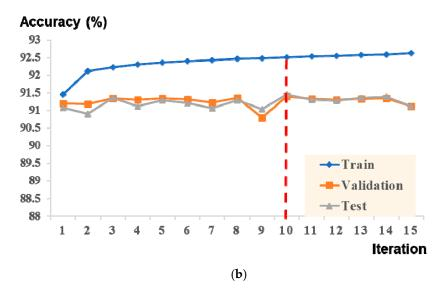
**Figure 4.** Evaluation of training times for best training accuracy. One iteration means that all the data samples in the entire training set have been used to train a deep learning model. (a) Training/validation/test accuracy trend for a single-epoch model. (b) Training/validation/test accuracy trend for a multi-epoch model.
