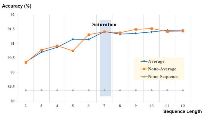
**Figure 3.** Performance of deep neural network model based on sequence length. The learning curve begins to plateau when more than 7 sequential epochs are used.
