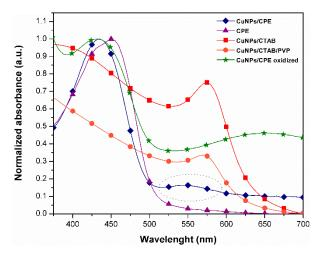
**Figure 1.** UV-vis spectra of the CPE and the copper nanoparticles (CuNP)/CPE (stabilized and oxidized), CuNP/cetyltrimethylammonium bromide (CTAB), and CuNP/polyvinylpyrrolidone (PVP)/CTAB composites in aqueous suspensions  $(10^{-4} \text{ mol} \cdot \text{L}^{-1})$ .
