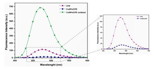
**Figure 2.** Fluorescence spectra of CPE and CuNP/CPE (stabilized and oxidized) composites in aqueous suspensions  $(10^{-6} \text{ mol} \cdot \text{L}^{-1})$ .
