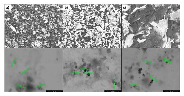
**Figure 3.** SEM (**up**) and FESEM (**down**) images of CuNP/CPE composites with different amounts of CPE: (**a**) 5 mg, (**b**) 15 mg, and (**c**) 30 mg.
