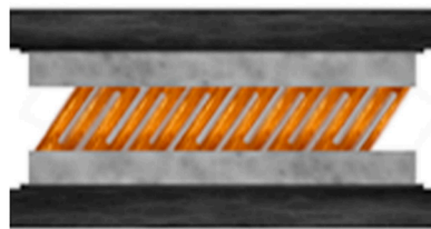
Figure 6. Low-temperature metallic gluing enabled by Ga- and In-coated nanorods [70].
