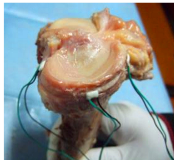
Fig. 1 The installment of strain gages at anterior, middle, and posterior part of the medial tibial plateau
