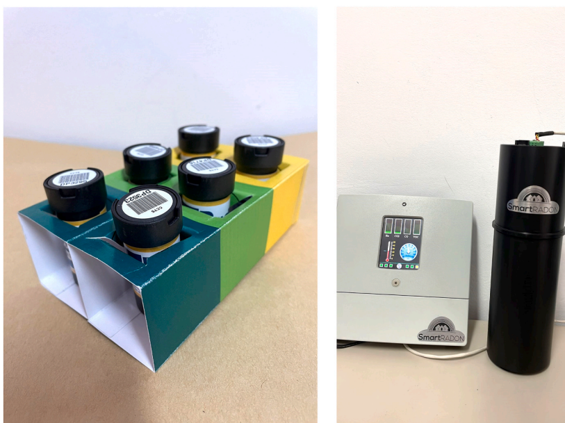
Fig. 1. Monitoring the IRC through passive method (CR-39 detectors, organized within the Lemon kit - left), respectively active method (ICA device - right).
