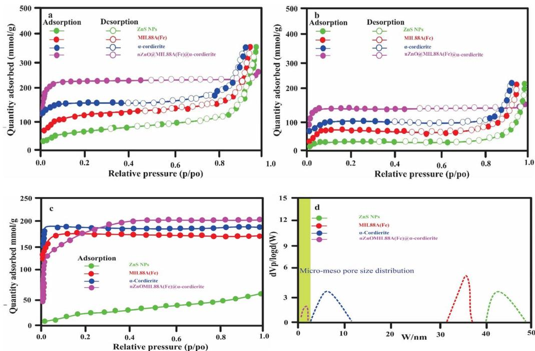
Fig. 5 N<sub>2</sub> adsorption–desorption plot of MIL88A(Fe) MOFs, ZnO NPs, α-cordierite porous ceramic, and nZnO@MIL88A(Fe)@α-cordierite composites before (a) and after (b) after desalination. (c) N<sub>2</sub> simulated sorption plot of MIL88A(Fe) MOFs, ZnO NPs, α-cordierite porous ceramic, and nZnO@MIL88A(Fe)@α-cordierite composites by NLDFT model. (d) Micro-mesopore size distribution for MIL88A(Fe) MOFs, ZnO NPs, α-cordierite porous ceramic, and nZnO@MIL88A(Fe)@α-cordierite composites.
