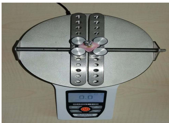
Figure 2 Biomechanical; reverse torque analysis, of the implants (Mark-10 Cap Torque Tester, Model TT01-12, NY, USA).
